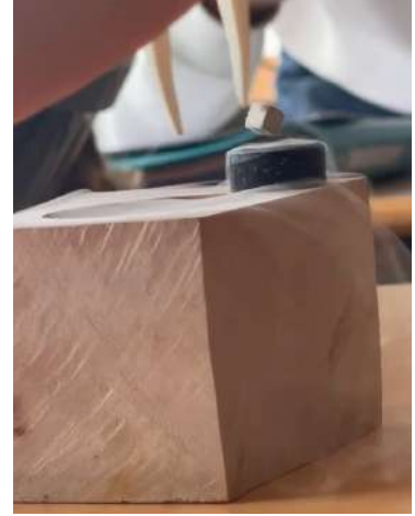
(c) When the magnet levitates, it can be perturbed a little with the tip of a tweezers without causing it to fall: the levitation is stable, which means, according to Earnshaw's theorem, that the magnetic properties of the ceramic at a sufficiently low temperature are not compatible with paramagnetism/ferromagnetism.
