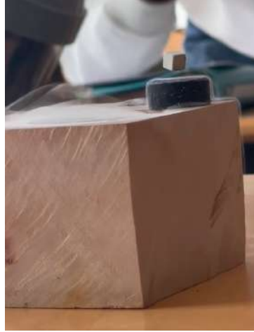
(b) A few seconds after pouring, the liquid nitrogen stops boiling, and the magnet lifts off the ceramic. The latter two are then removed from the cryostat to make the levitation easier to visualize. Note again the white fumes exhaling from the ceramic, due to the solidification of ambient water vapor near the cold ceramic.
