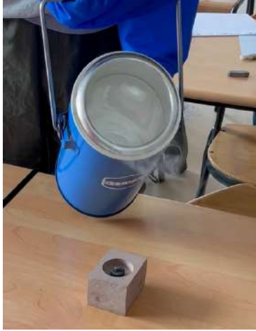
(a) Overview of the experimental setup: liquid nitrogen lies in the Dewar storage (blue), while the magnet (metallic) is placed on top of the ceramic button (black), the two later being placed in the cryostat (beige). The white fumes are due to the solidification of water vapor when it comes into contact with cold nitrogen vapor.
